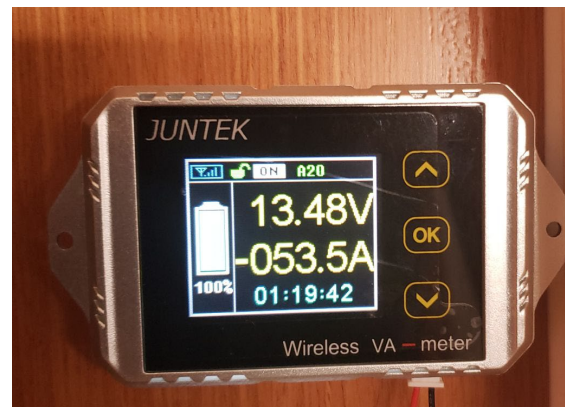
Fig. 16.14: Measuring device for the solar charging current.
