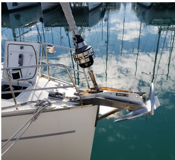
Fig. 8.6.: Our new anchor (Rocna 33kg).
