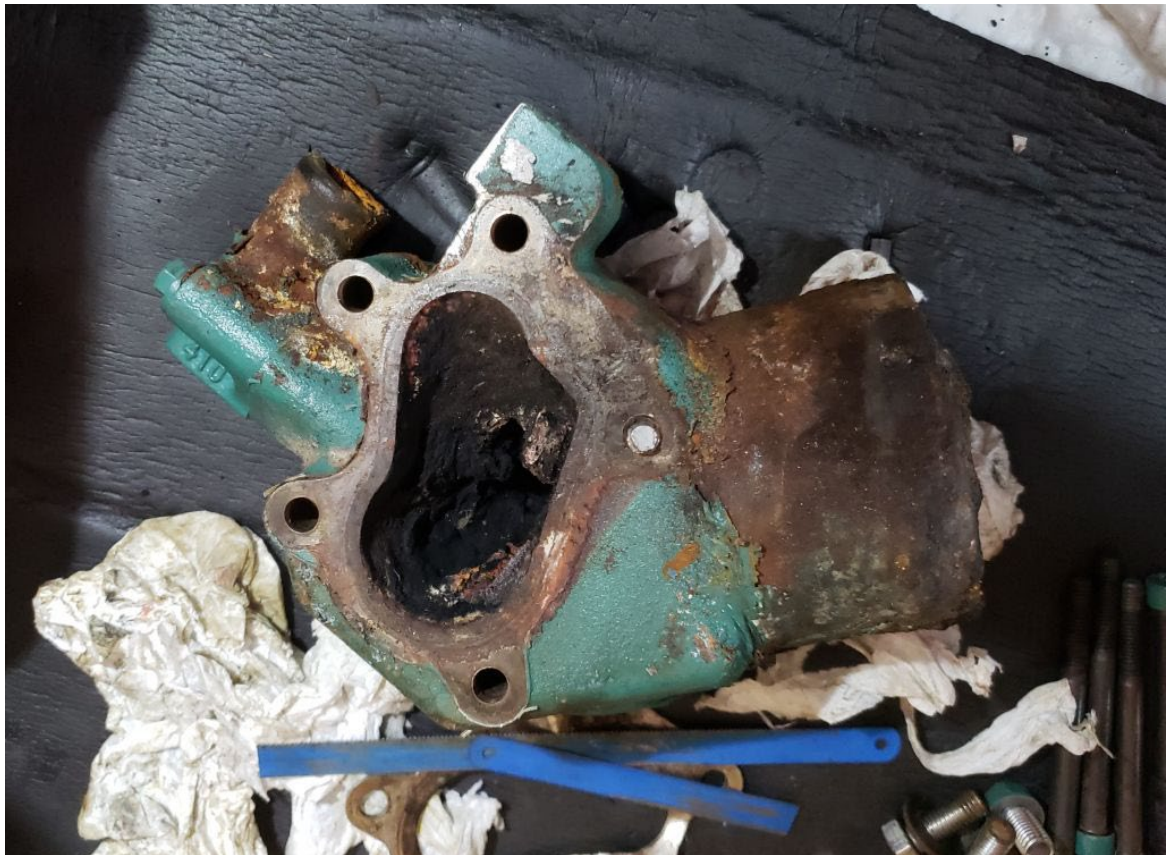
Fig. 26.12: The rusted-through exhaust manifold of our Volvo.
