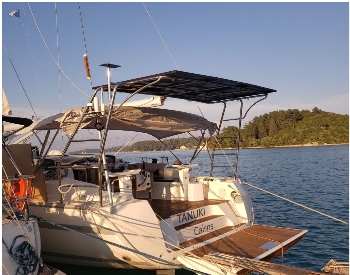
Fig. 16.5: Gantry attached to the hull and solar panels mounted.
