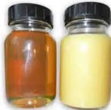
Fig. 51.6: Oil contaminated with water looks milky white (right).
