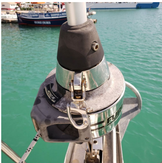
Fig. 16.25: Our Furlex. Somewhat weathered but mechanically in good condition.
