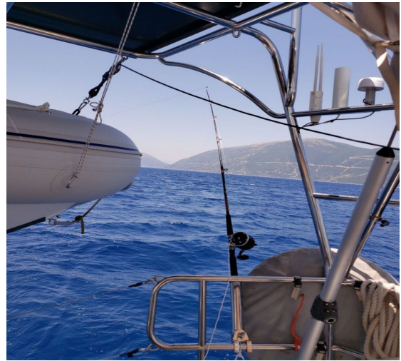
Fig. 16.18: Pulleys to hoist the dinghy up the equipment carrier.
