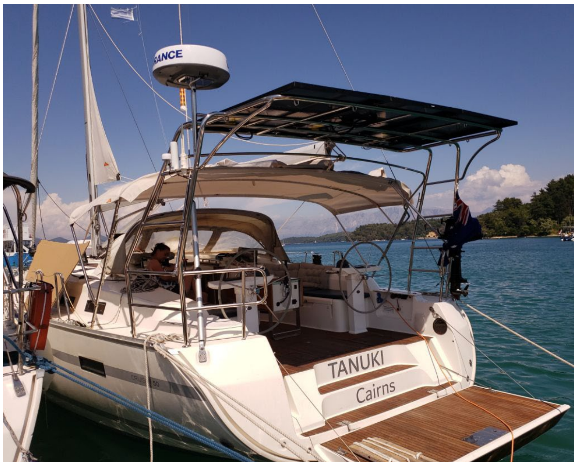
Fig. 16.6: Almost finished. Wired, radar mounted and rear railing welded on.
