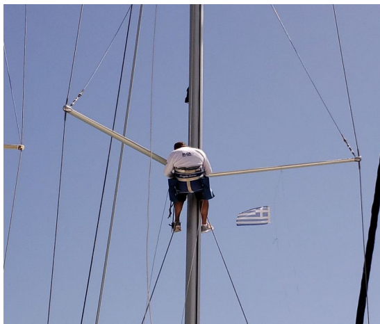
Fig. 16.21: New spreader on. Done!
