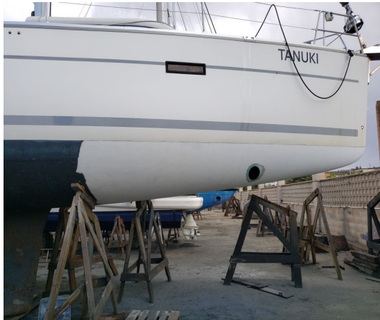
Fig. 26.5: The old antifouling is being sanded off (first day).
