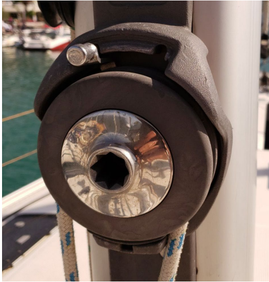
Fig. 16.23: Clamping disc of the main furler.
