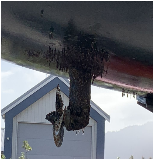
Fig. 54.28: Saildrive and propeller have some (, a lot!) of fouling.
