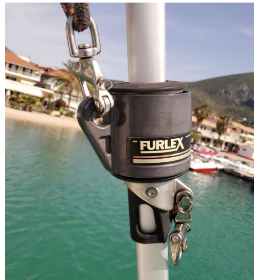
Fig. 16.26: The upper part of the roller system.
