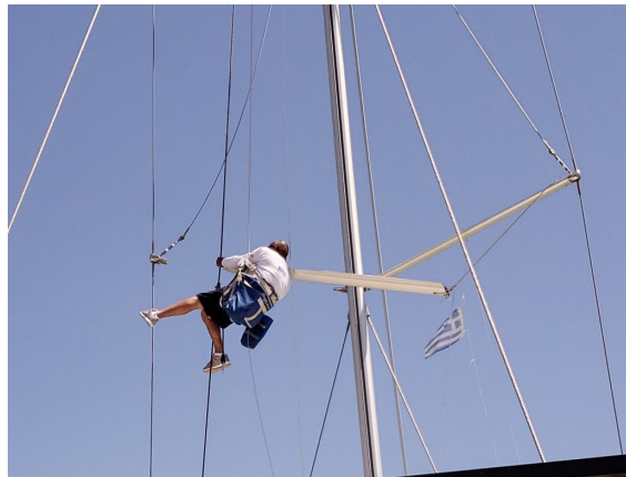
Fig. 16.20: The spreader is being removed.
