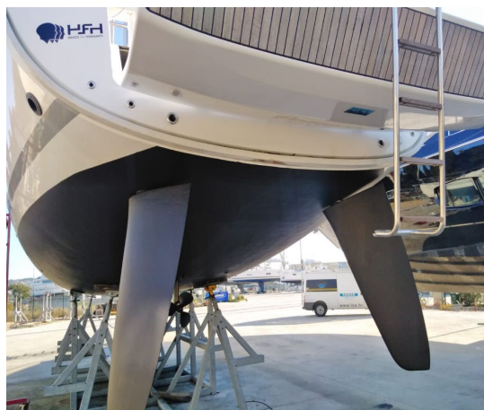
Fig. 5.3: Twin rudder system.
