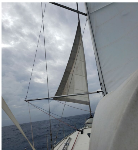
Fig. 31.1: Our genoa (here heavily reefed) is poled out at port with the whisker pole.
