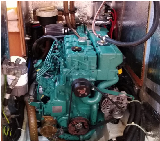
Fig. 5.6.: The engine (Volvo D2-75).
