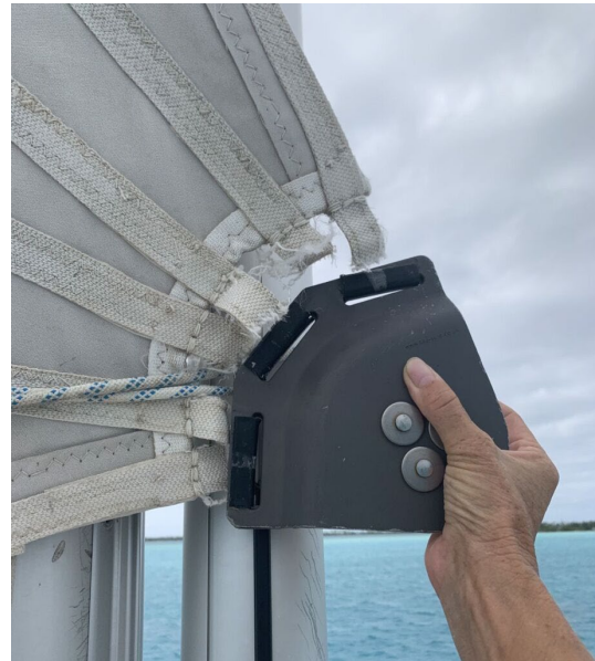
Fig. 43.2: The pulley on our mainsail has torn out.
