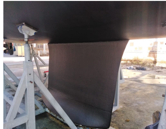
Fig. 4.8: Underwater hull freshly painted, keel still attached.
