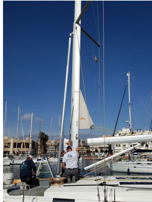
Fig. 26.29: The new spinnaker pole to be stored on its mast track.
