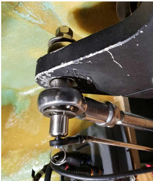
Fig. 29.9: Our new bolt, already installed.
