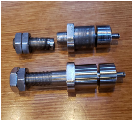
Fig. 29.7: AP-bolts, broken versus new.
